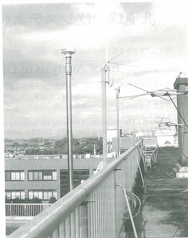
Fig. 1-2 UNCT site. From this side, UNCT (GPS 17N) and DGPS beacon receiver built in H-field antenna (GBR 23).
