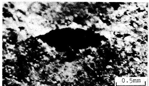
(b) controlled by \dot{J} (small crack)
