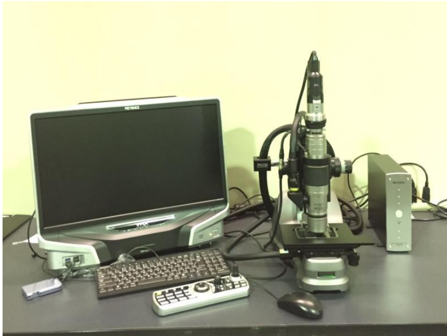
Fig. 3.3.4 Digital microscope for fiber diameter measurement
