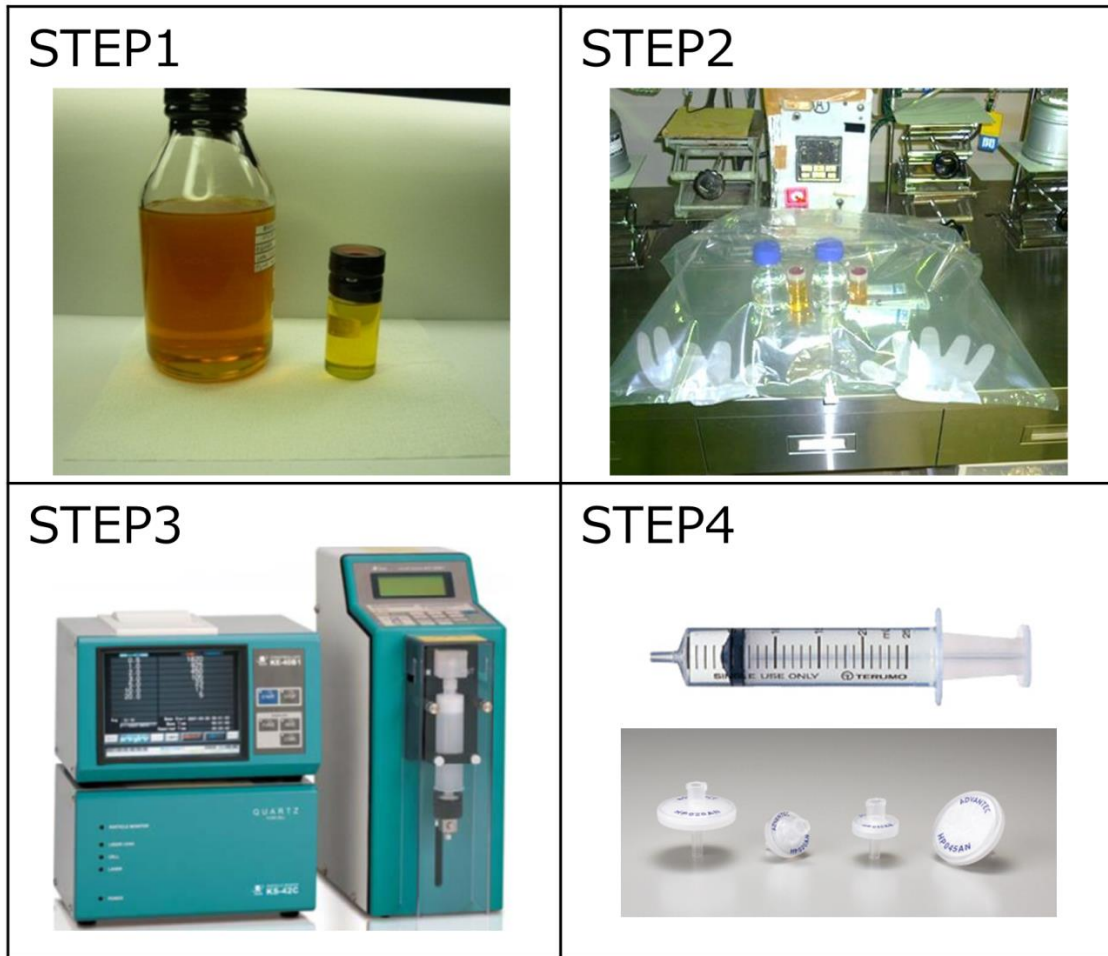
Fig. 4.3.19 Procedure for particle measurement in raw material polymer
