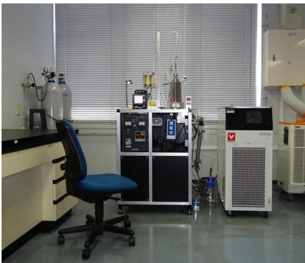
Fig. 6.2.2 Appearance of electric furnace
