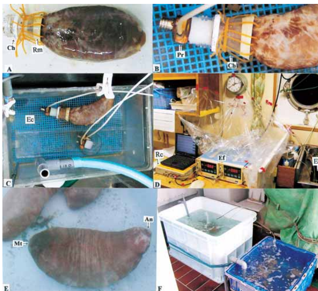
Fig. 1. Experimental system (A-D) and condition stocked a sea cucumber, Molpadia roretzi , into reservoir tank (E and F). Ch; small chamber for collecting ventilated water, Rm; rubber membrane, Pr; probe of electromagnetic flowmeter, Ec; experimental chamber, Rc; recorder (MacLab system), Ef; electromagnetic flowmeter, Mt; mouth, An; anus.
