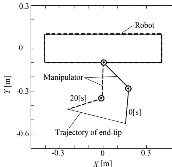
(a) Motion of underwater robot manipulator
