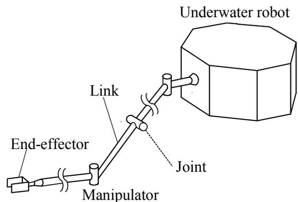
Fig. 1. An example of an underwater robot manipulator.
