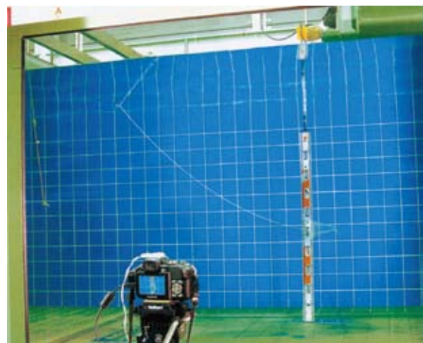
Fig. 4. Photographing of the position of the lead cord end by a digital camera.
