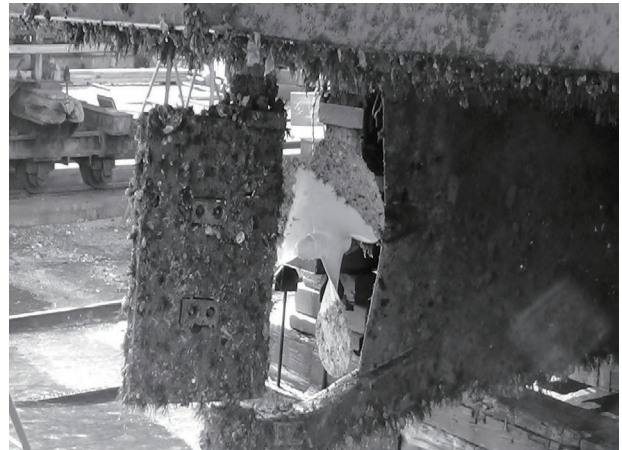
Photo2-2 Condition of rudder and propeller before cleaning
