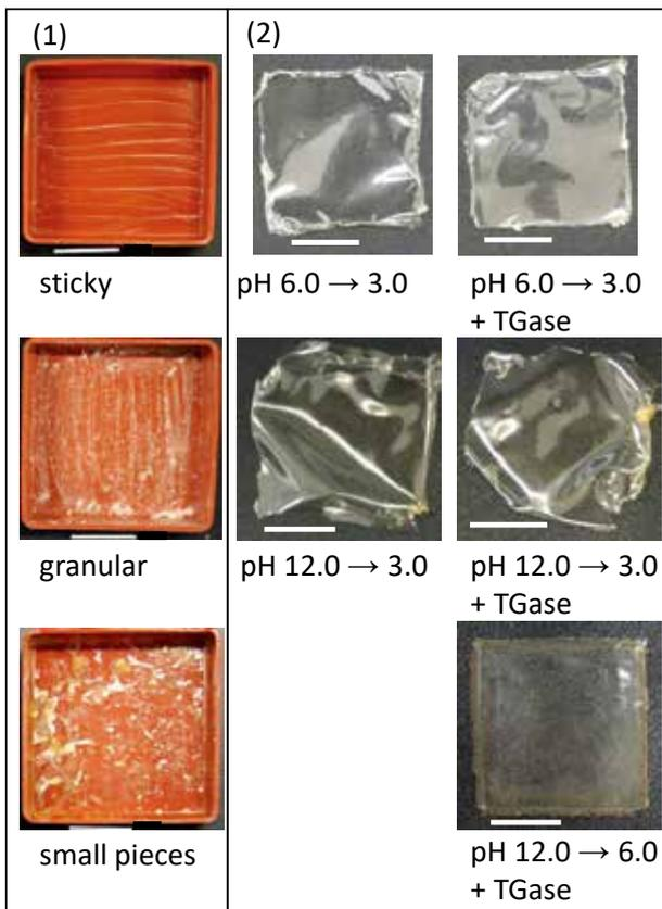
**Fig. 1** Dried salvages of each film-forming condition from water-soluble protein of Walleye pollock roe. (1) Typical appearance of non-film like salvages. (2) Film-like salvages of each condition (extraction pH → adjusted pH + transglutaminase (TGase)). White bars showed 20 mm.
